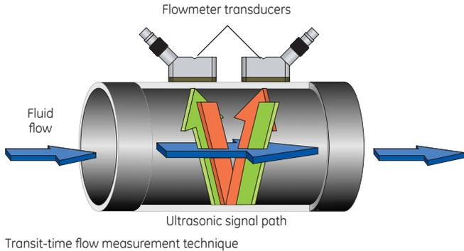
In this method, two transducers serve as both ultrasonic signal generators and receivers. When mounted on a pipe, they are in acoustic communication with each other, meaning the second transducer can receive ultrasonic signals transmitted by the first transducer and vice versa.
